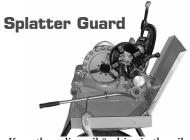
•Keep threading oil & chips in the oiler and off the walls and floor.
