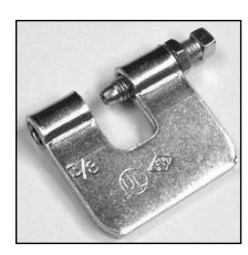
Designed for attaching hanger rod to the bottom flange of a beam. the hanger rod should make contact with the beam flange to ensure full engagement.
