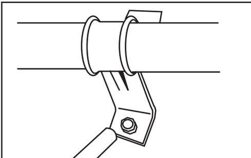
3. Fasten the strap to the wood surface using the two hex head screws provided.
