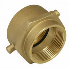
This 2-1/2 in. NPT x NST Cast Brass Snoot & Swivel secures to an FDC's inlet to allow fire hose to pump water into an inlet body. These Cast Brass finished 2-1/2 in.
