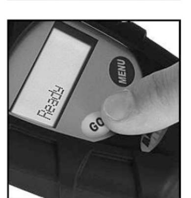
Press and release <GO> to automatically zero the instrument. Remember to clean and dry the measuring surface after calibration.
