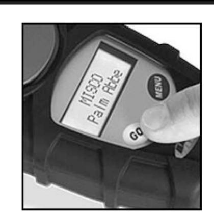
Press and release <GO> to turn the instrument on.
