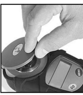
Close the sample cover and allow some time for the temperature to equalize. The sample cover MUST be closed to calibrate or take readings.
