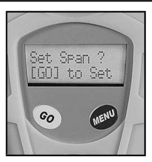
The Span Point represents a calibration point toward the upper end of the Palm Abbe range. Although it is important to Zero Set the Palm Abbe daily, you may at some time want to set the span adjustment as well. The span should be set if you notice a general degradation of the instrument's accuracy and precision and/or on a periodic basis determined by your particular history with the instrument.
