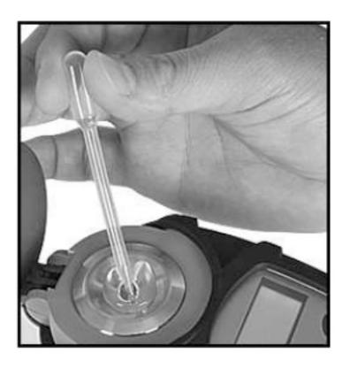
Inspect the measuring surface to make sure it is clean and dry. Place a few drops of distilled water on measuring surface.
