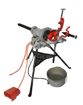
Reversible 1/2 HP universal motor. Capacity: 1/8"-2" (3mm-50mm) pipe On/Off/Reverse switch.
