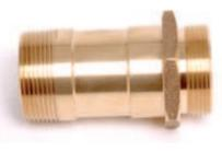
Male to Male Hose rack nipple used with swinging hose rack. Same size both ends. Male NPT x Male NST thread.
