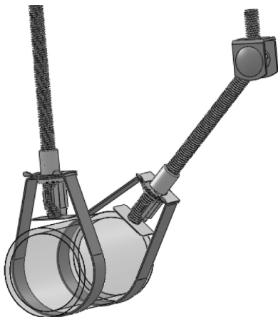
BRANCH LINE RESTRAINT NFPA13 2010 Section A.9.3.6.1(5)
