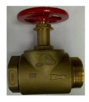
Heavy Duty 2-1/2" (65 mm) straightway hose valve, 300 lb (2070 KPa) pressure tested. Lightweight cast brass body with Forgeline Bonnet and Seat Assembly.
