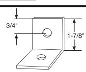
Designed for use with wood, steel or concrete beams to provide a means for supporting hanger rod.
