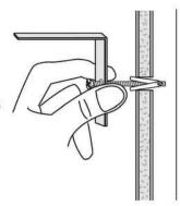
Pull back on assembly to hold the wings inside the wall to prevent the wings from spinning while tightening bolt. Turn the bolt with the screwdriver until firmly tightened.
