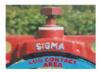
The SIGMA ONE-LOK Series SLCE is a mechanical joint restraining gland that implements a series of individually activated wedges into the mechanical joint follower gland. When the wedge segment is engaged by the actuating bolt, the primary contact edges of each wedge segment lock onto the pipe wall. This action causes the primary contact edges to grip the pipe and effectively restrain all classifications of both AWWA C900/C905 and ASTM D2241 IPS size PVC pipe.
