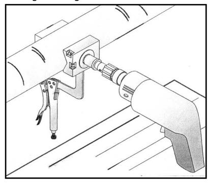
Complete with clamp with levels, six hole saw guides, six Lenox® holesaws, two Lenox® arbors, pilot bit, carrying case.
